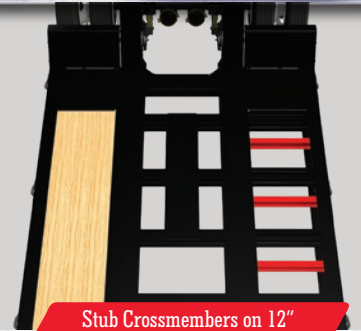
Stub Crossmembers on 12" Centers for Maximum Floor Life
