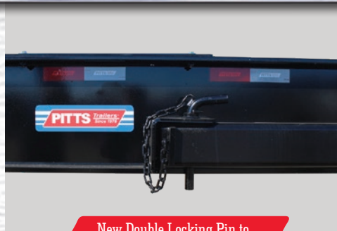
New Double Locking Pin to Secure Pull Bar
